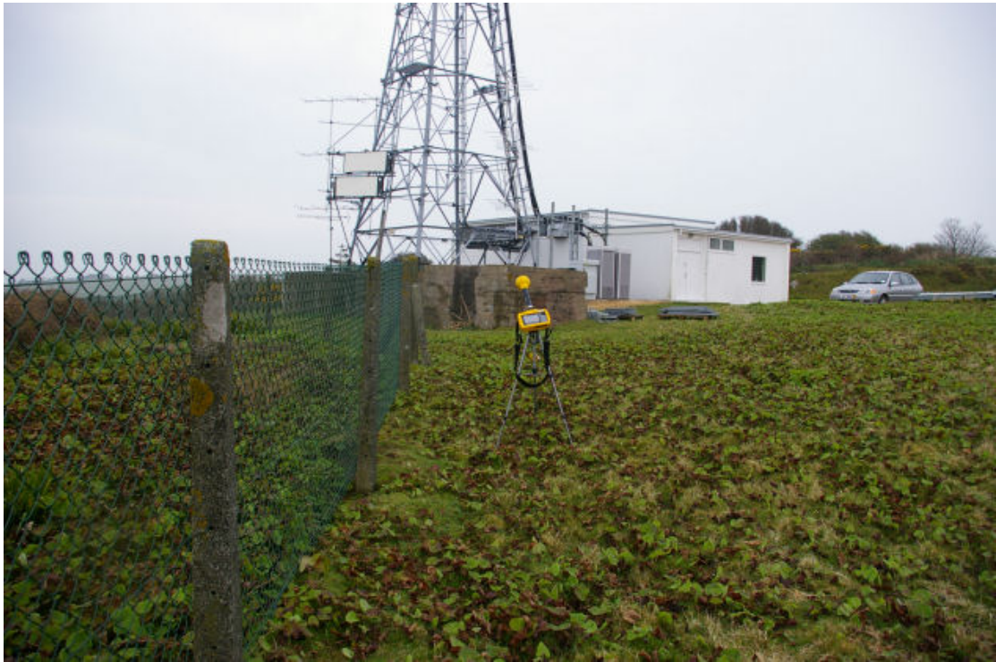
Figure 5 – EM Probe at the Arqiva site – Loc 27 (900 peak and Wave UMTS Peak)
