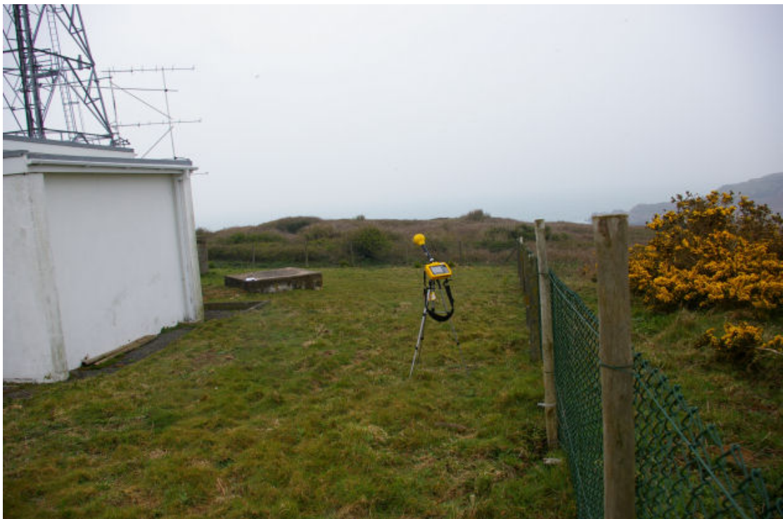
Figure 6 – EM Probe at the Arqiva site – Loc 12 (1800 peak and Airtel UMTS peak)
